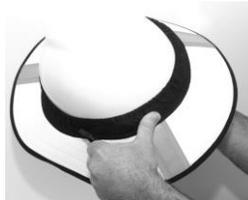
**Step 5.** Check for correct installation. Centers of hard hat and visor should align; if necessary, pull to straighten. Check for a secure installation by gripping the visor on both sides and shaking the hard hat. The product should not be loose or detach from the hard hat. If the product does not seat as described herein, do not use the Da Brim PRO Vision visor with this hard hat.
